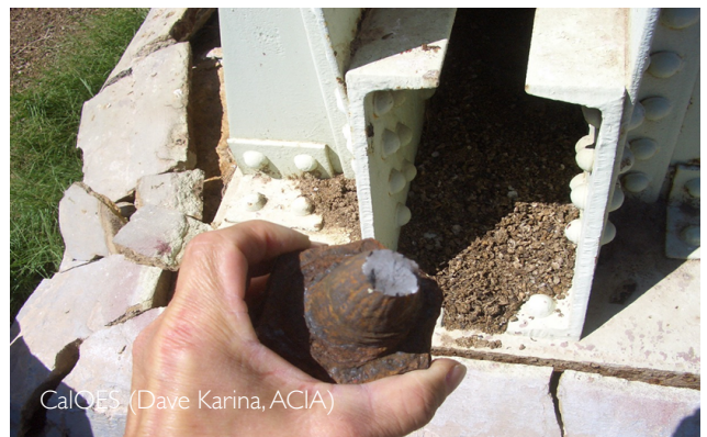
Left: El Centro Water Tower Bolt Fracture
