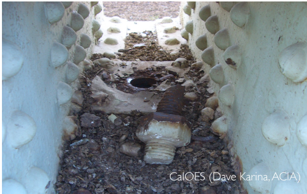
Left: El Centro Water Tower Bolt Fracture
